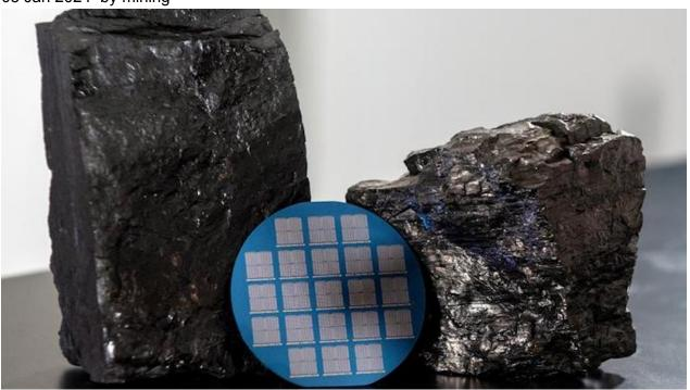
A wafer containing memristors fabricated with high-quality two-dimensional carbon processed from bituminous Blue Gem coal mined in southeastern Kentucky, two samples of which are shown here. (Image by the Grainger College of Engineering at University of Illinois Urbana-Champaign).
