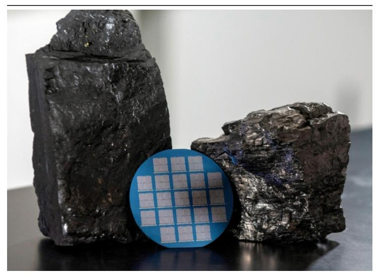
A wafer containing memristors fabricated with high-quality two-dimensional carbon processed from bituminous Blue Gem coal mined in southeastern Kentucky, two samples of which are shown here. Credit: The Grainger College of Engineering at University of Illinois Urbana-Champaign
