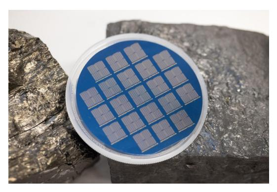
A 3-inch wafer with over 15,000 field effect transistors fabricated with carbon material derived from coal.
