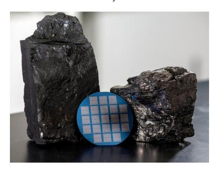
A wafer containing memristors fabricated with high-quality two-dimensional carbon processed from bituminous Blue Gem coal mined in southeastern Kentucky, two samples of which are shown here. (Image: University of Illinois Urbana-Champaign)
