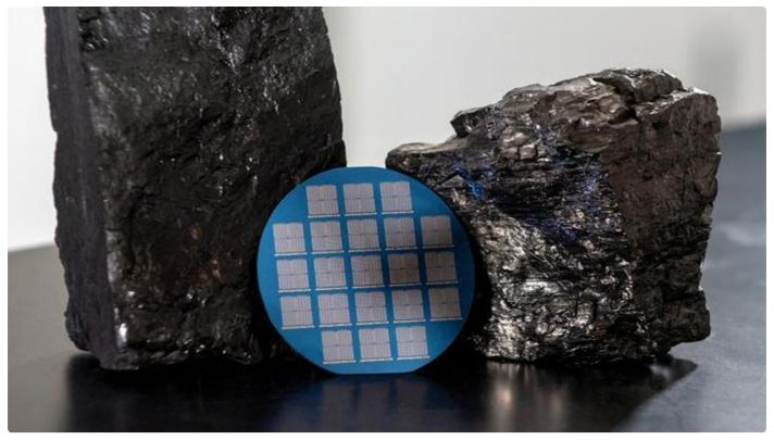
A wafer containing memristors fabricated with high-quality two-dimensional carbon processed from bituminous Blue Gem coal mined in southeastern Kentucky, two samples of which are shown here. Credit: The Grainger College of Engineering at University of Illinois Urbana-Champaign.
