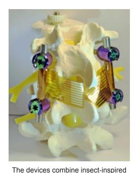
nanostructured foils with highly sensitive flexible electronics. Here the device prototypes are applied to commercially available spinal implants and displayed on a spine model.
