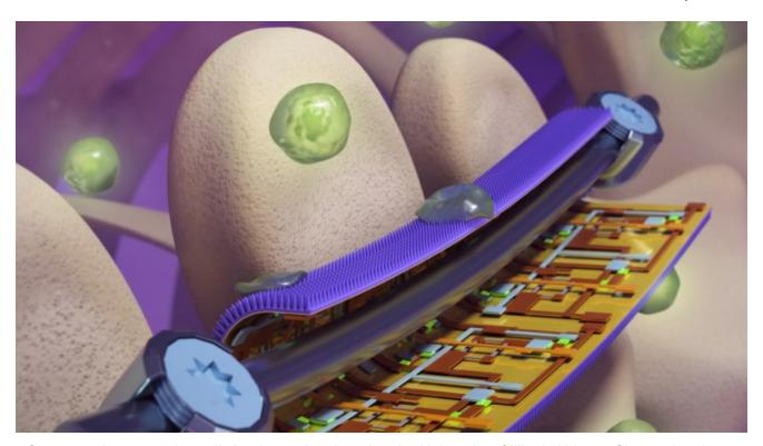
Smart coatings on orthopedic implants, developed at the University of Illinois Urbana-Champaign, have bacteria-killing nanopillars on one side and strain-mapping flexible electronics on the other. This could help physicians guide patient rehabilitation and repair or replace devices before they fail. Image by Beckman Imaging Technology Group
