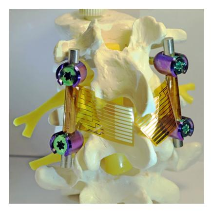
The devices combine insect-inspired nanostructured foils with highly sensitive flexible electronics. Here the device prototypes are applied to commercially available spinal implants and displayed on a spine model.
