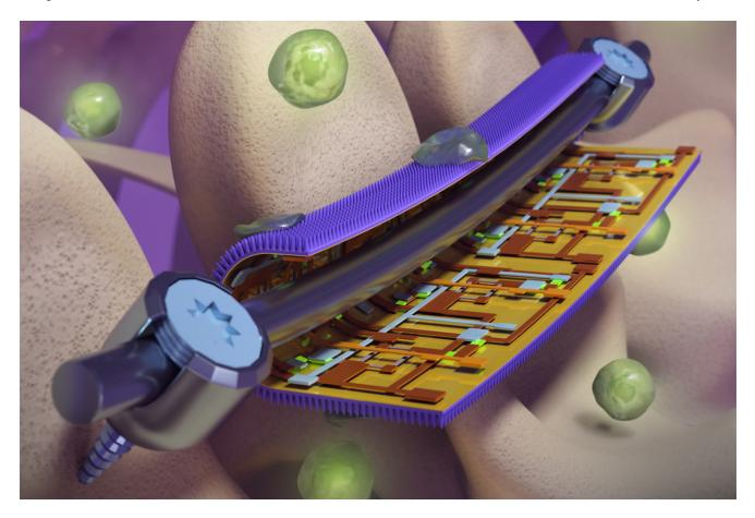
Smart coatings on orthopedic implants, developed at the University of Illinois Urbana-Champaign, have bacteria-killing nanopillars on one side and strain-mapping flexible electronics on the other. This could help physicians guide patient rehabilitation and repair or replace devices before they fail.
