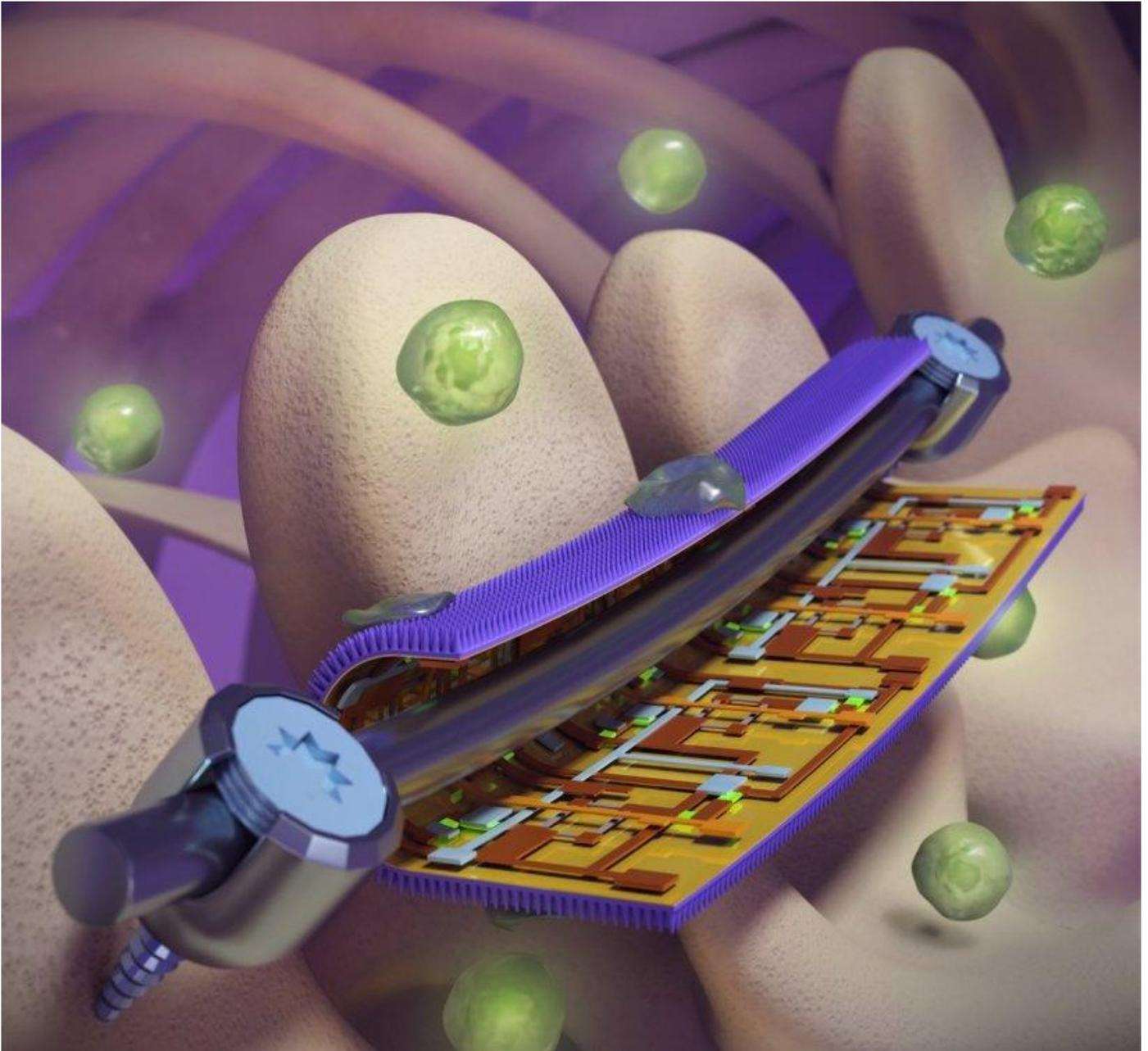
*Smart coatings on orthopedic implants, developed at the University of Illinois Urbana-Champaign, have bacteria-killing nanopillars on one side and strain-mapping flexible electronics on the other. This could help physicians guide patient rehabilitation and repair or replace devices before they fail.*
