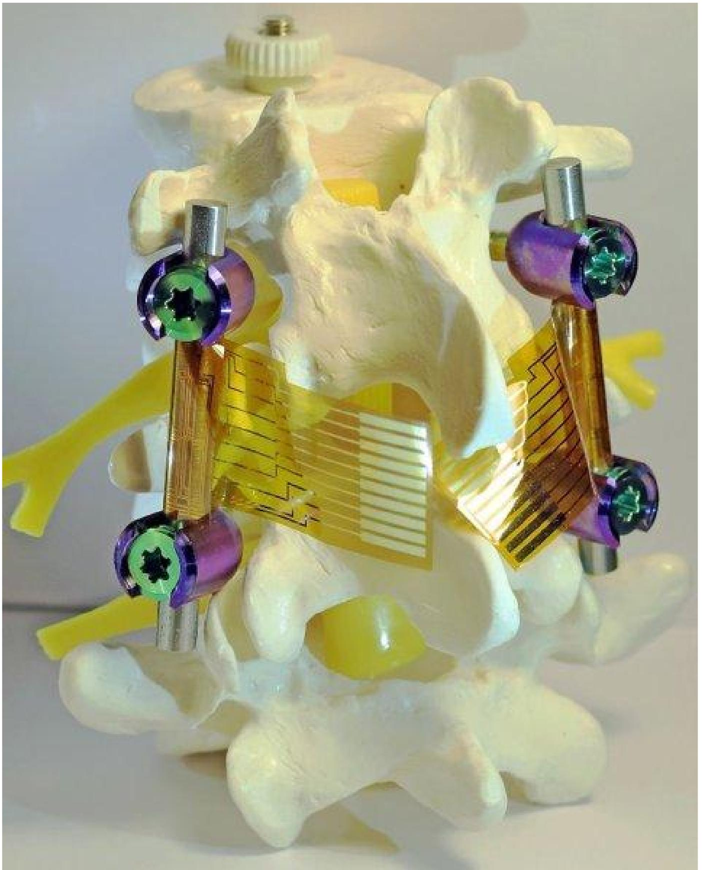
*The devices combine insect-inspired nanostructured foils with highly sensitive flexible electronics. Here the device prototypes are applied to commercially available spinal implants and displayed on a spine model.*
