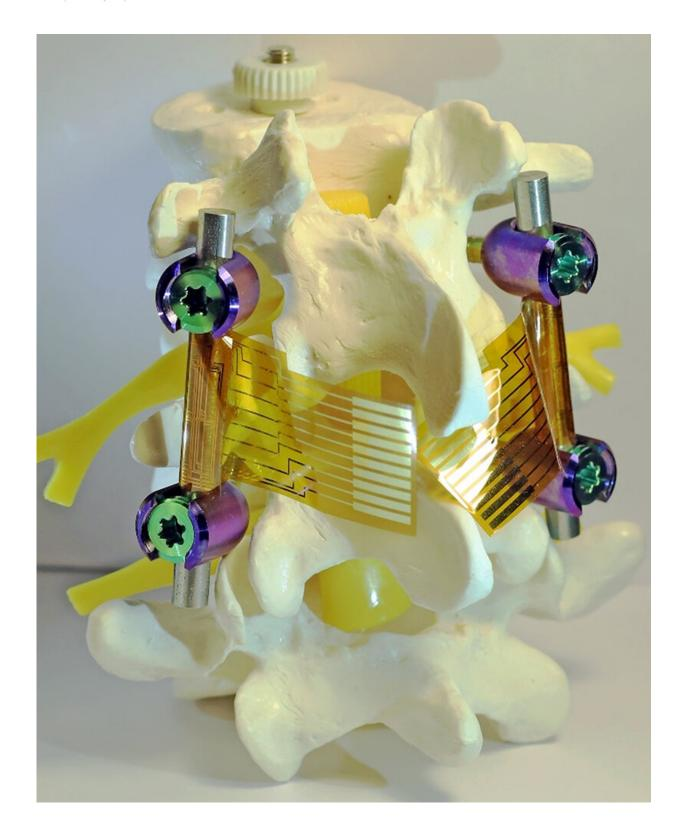
The devices combine insect-inspired nanostructured foils with highly sensitive flexible electronics. Here the device prototypes are applied to commercially
