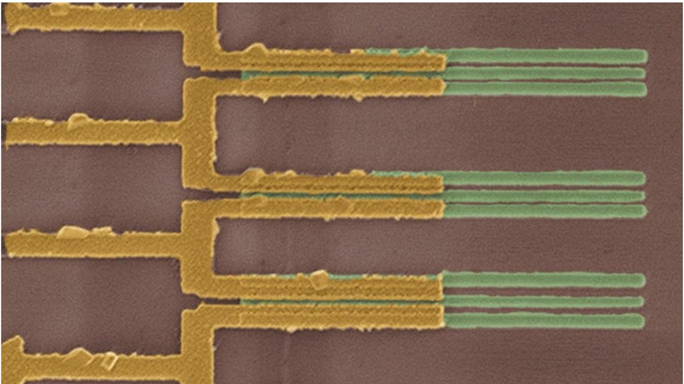
Carbon nanotube transistors (seen here in green) are fed electricity by metal contacts (yellow).
