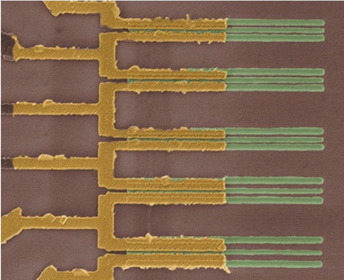
This microscopic view shows a faint vertical line consisting of carbon nanotube segments bonded to the golden-colored parallel wires. IBM Research
