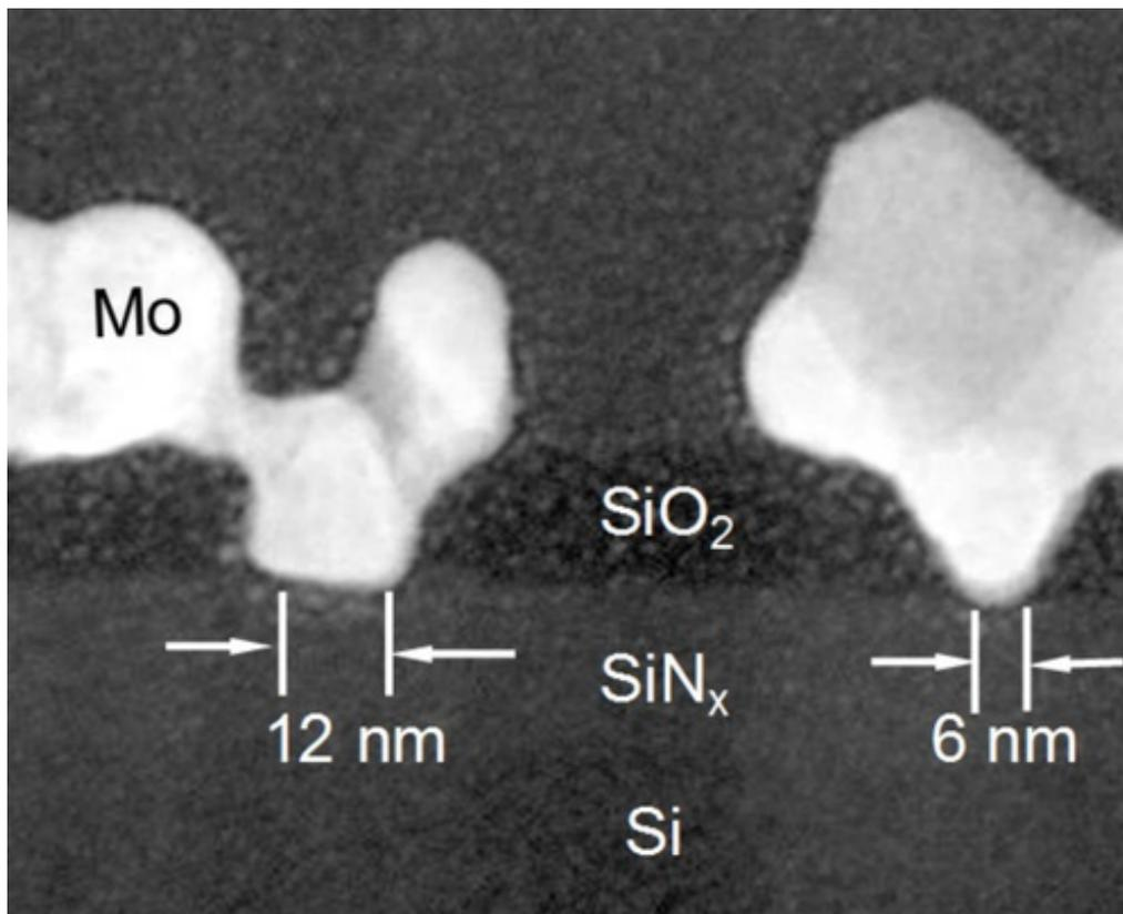
Cross-sectional transmission electron microscope (TEM) image showing the fabricated nanotube transistor with an end-bonded contact.
