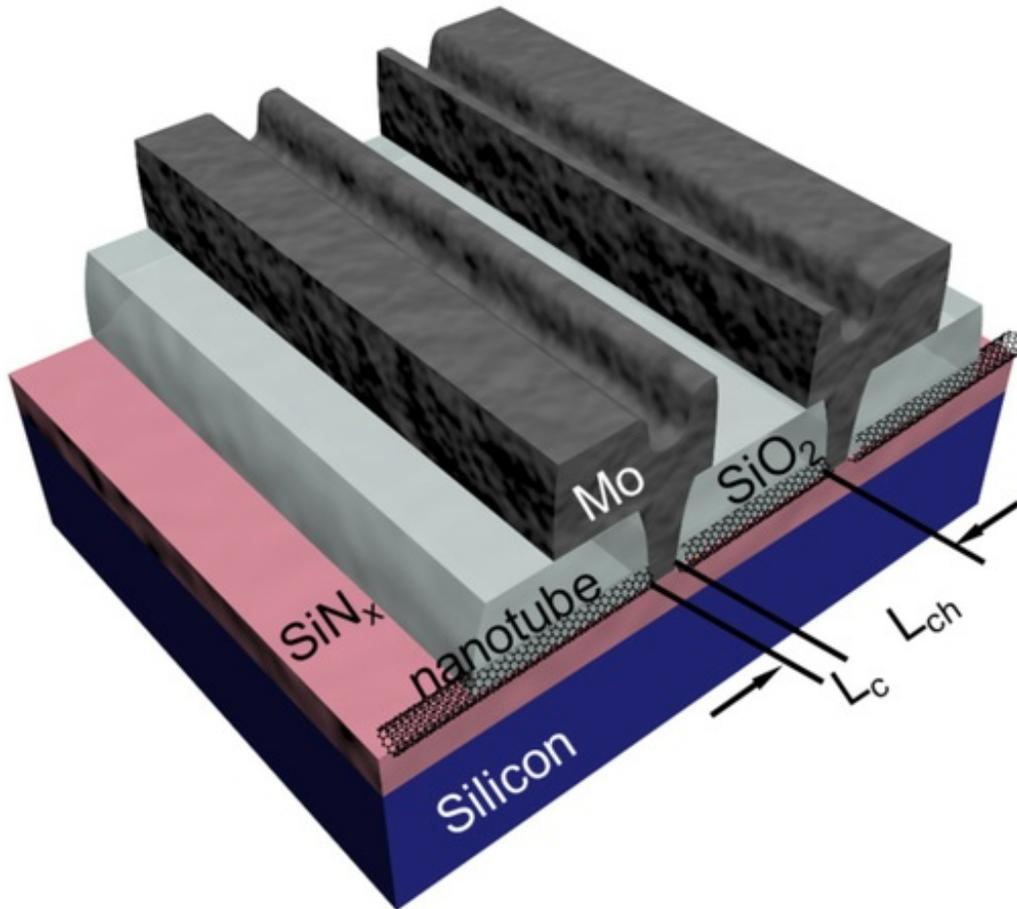
Schematic showing the fabricated nanotube transistor with an end-bonded contact and a contact length below 10 nm.
