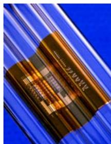
The so-called "nanonet" technology—circuits made of numerous carbon nanotubes randomly overlapping in a fishnet-like structure—has been plagued by a critical flaw: The network is contaminated with metallic nanotubes that cause short circuits.
