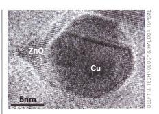
at high temperature in hydrogen, the team directly observed the growth, structure, and evolution of copper nanocrystals with angstrom resolution on a subsecond timescale.
