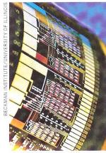
Networks of carbon nanotube transistors result in high-powered, lightweight, flexible integrated circuits.
